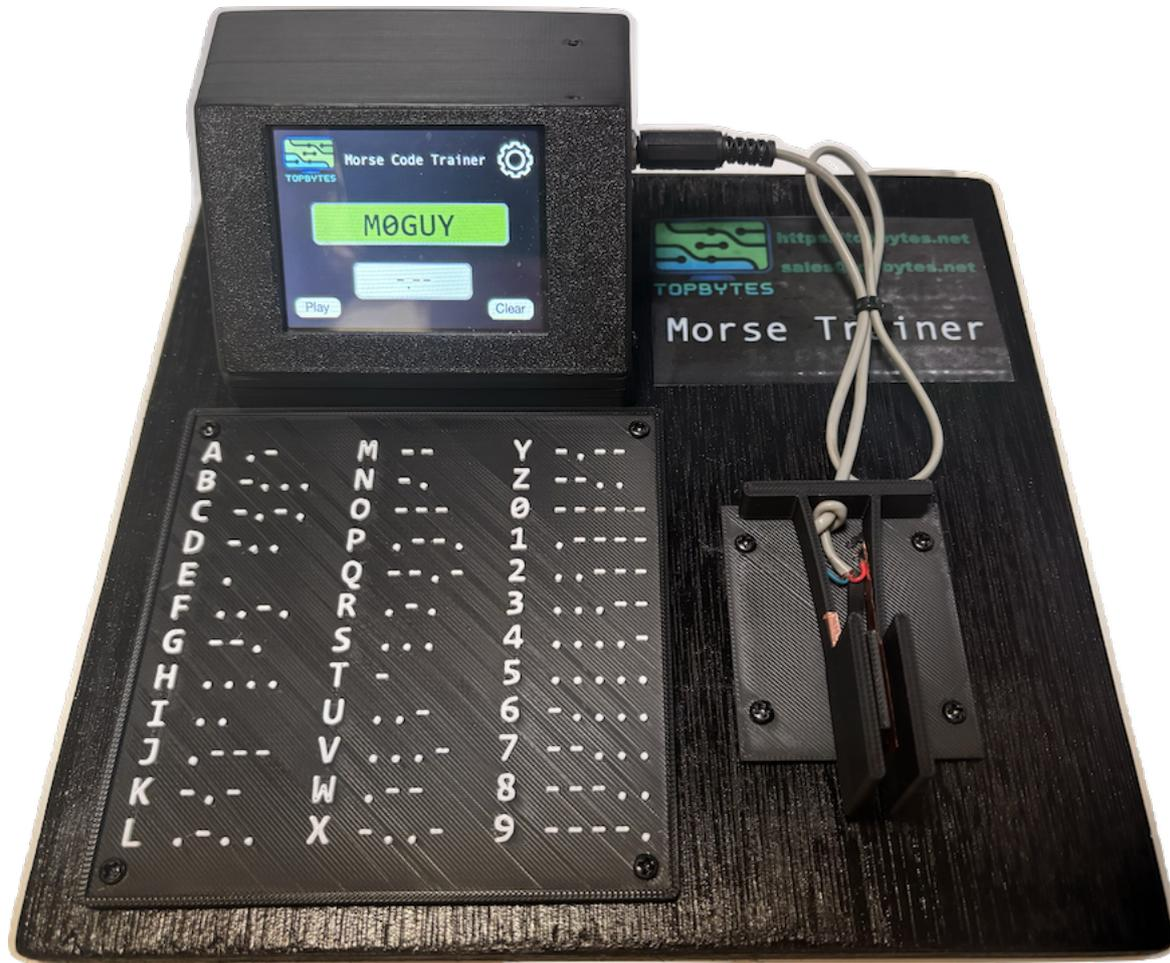
Fig. 4: NRC demo unit with paddle and morse reference chart
