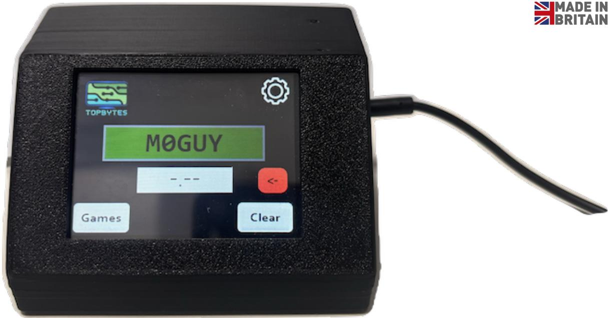
TopBytes Morse Trainer. Small portable battery powered device to help with learning to send and receive morse code. Connect your own straight key or morse paddle using a *standard 3.5mm stereo plug*.
